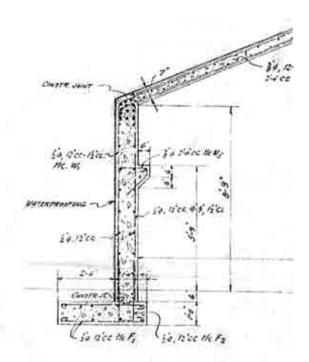
FIGURE 89. Detail from original construction drawings showing presumed section through main concrete shell. See Appendix A for entire sheet. (OCMU Coll.)
