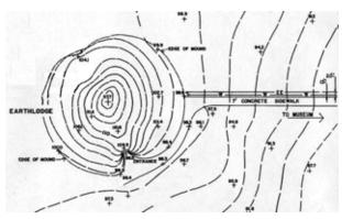
**FIGURE 79.** Topographical plan of Earth Lodge and vicinity, drawn 1974. SInce the mound was reconstructed in 1975, the mound may differ slightly from this drawing. (OCMU Coll.)
