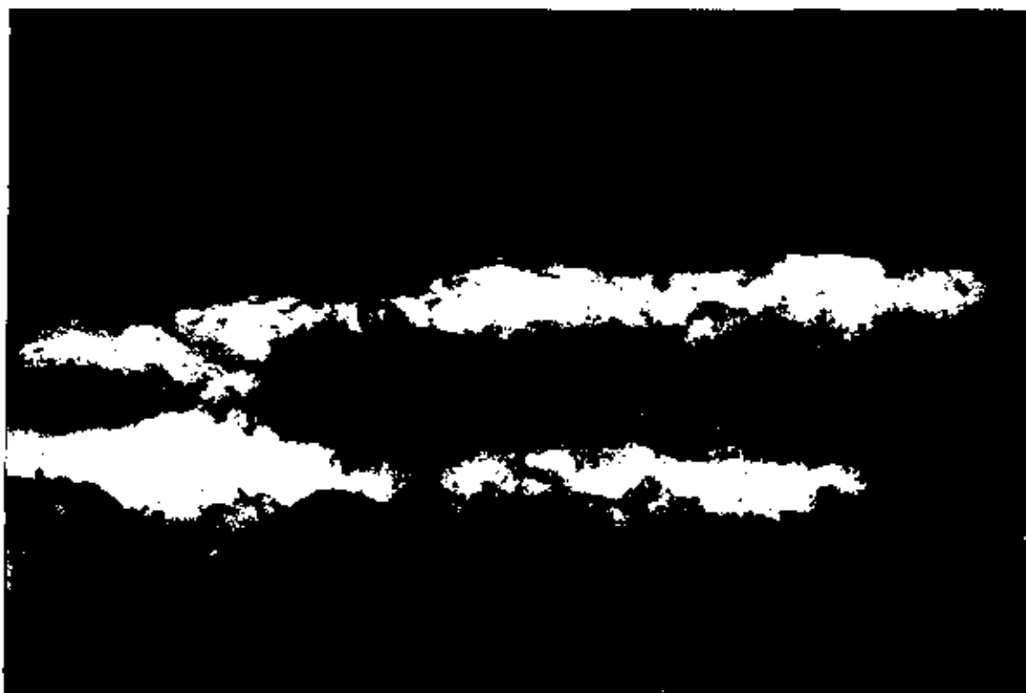
Photograph P37. This photograph was taken through a fluorescence microscope of a remnant of the original graining on the door between Room 109 and Hall 111. Over the light-rose basecoat can be seen the graining glaze. The color shift in the paint layers is the reaction of the oil binders to the ultraviolet radiation. 200X magnification. Exciter filter - BG12. Barrier filter - GG475.
