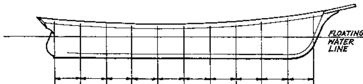
DIVIDE LENGTH OF HULL AT FLOATING WATER LINE INTO EVEN NUMBER OF EQUALLY SPACED INTERVALS (10 IS COMMON)
