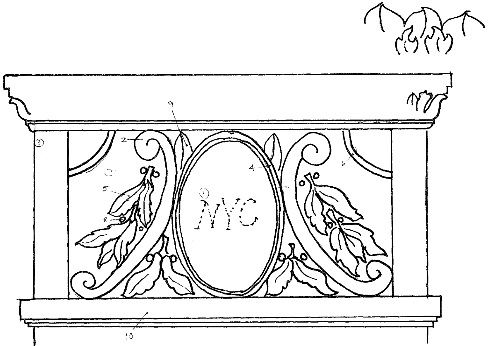
Figure C-3. Schematic drawing of ornamental plasterwork found on all pier capitals at the second floor level of the lobby.
