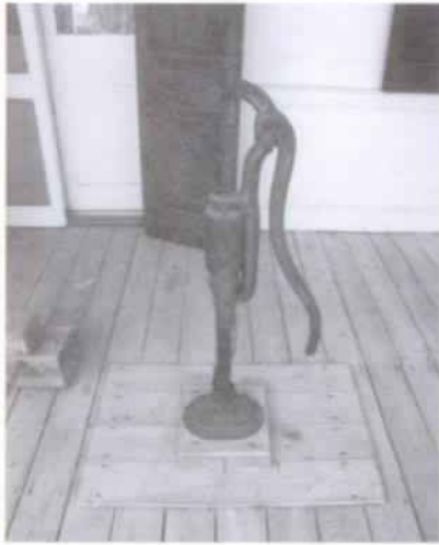
Figure 48 Myers pump on rear gallery, still connected to cistern located below. (NPS-SERO-CRS, 2001)
