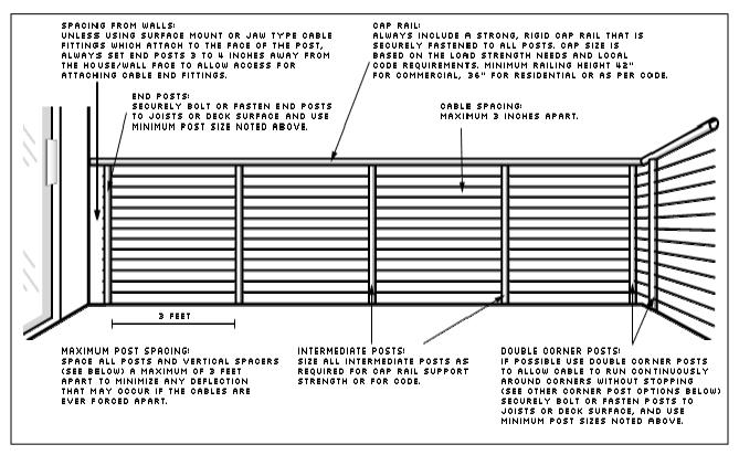
Example of a tension cable fence with double corner posts and no foot rail (Feeney Gateway, http://www.cablerail.com/index\_2.html).
