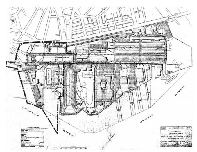
Figure 5.16: Digitally enhanced plan for the yard in 1902-03 showing the new bulkhead line with the existing piers extended, Dry Dock 2 under construction, and relocation of Buildings 10. Current park boundary is outlined (Courtesy of Boston NHP Archives).
