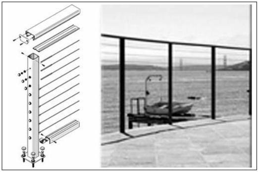
Examples of tension cable fencing. Left: schematic drawing; Right: unobstructed views of a harbor through a fence (Feeney Gateway, http://www.cablerail.com/index\_2.html).
