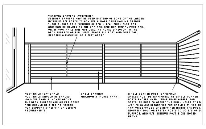
Example of a tension cable fence with a single corner post and a foot rail (Feeney Gateway, http://www.cablerail.com/index\_2.html).
