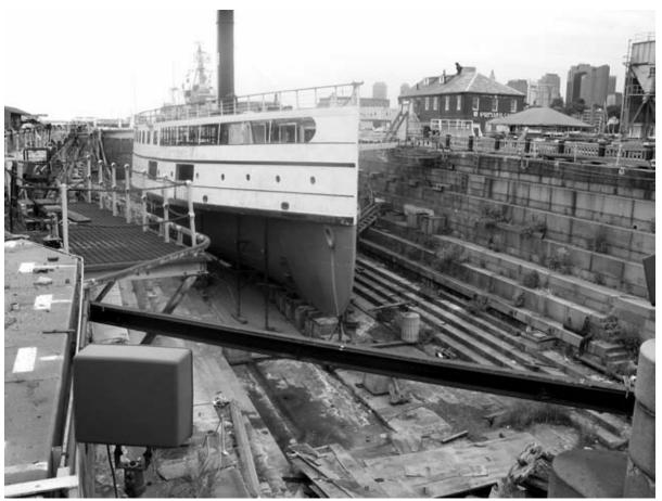
Figure 9.8: Dry Dock 1 and the SS Nobska looking south with Pier 1 and the Boston skyline to the right. The ship rests on keel blocks and is stabilized by the vertical shoring (OCLP, 2003).
