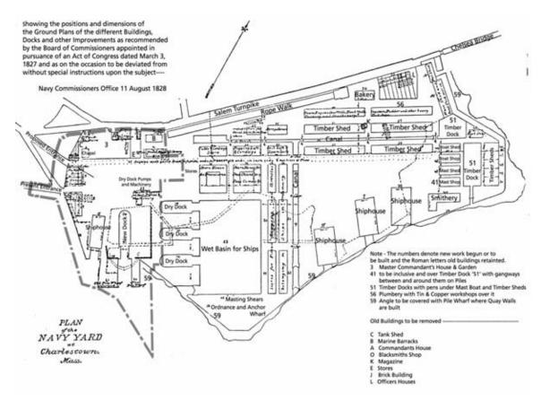
Figure 3.1: Digitally enhanced plan of the yard showing existing conditions and proposed additions, 1828. Current park boundary is outlined (from Prebble, 1875).
