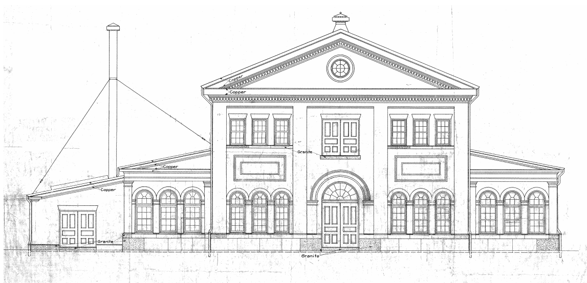
Figure 5: East elevation shown in construction drawings (2/08/04). Note that the gable roof has been rotated 90° to align the pediment with the east façade. Windows have also been changed from 9/9 to 6/6, with half-round transoms on the first floor windows.
