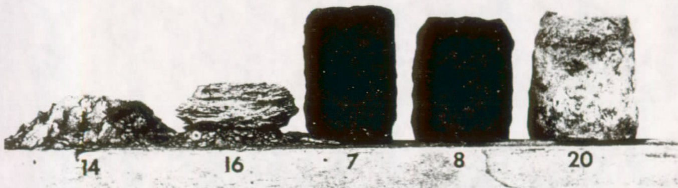
FIGURE 7. Selected cylinders subjected to freeze-thaw test. Nos. 14 and 16, with 10 and 12 percent cement by volume respectively, failed at the third cycle. Both were made up with equal parts clay and silt-loam. No. 20, with 15 percent cement by volume, is shown at the 12th cycle. Nos. 7 and 8, consisting of three parts clay, two parts silt-loam, and emulsified bitumen, were tested in conjunction with the soil-cement and are shown at the 15th cycle.
