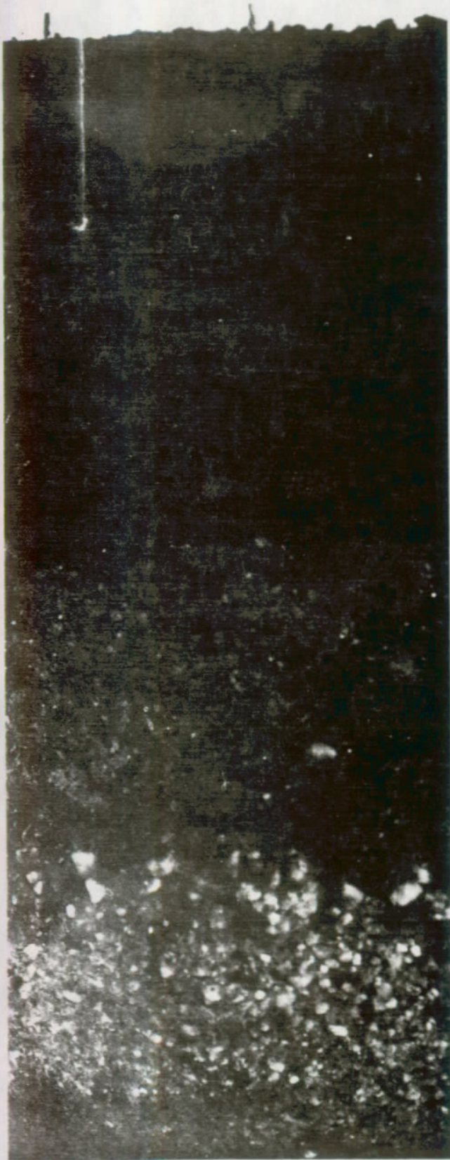
FIGURE 12. A close-up view of a well graded soil after suspension in water and settling.
