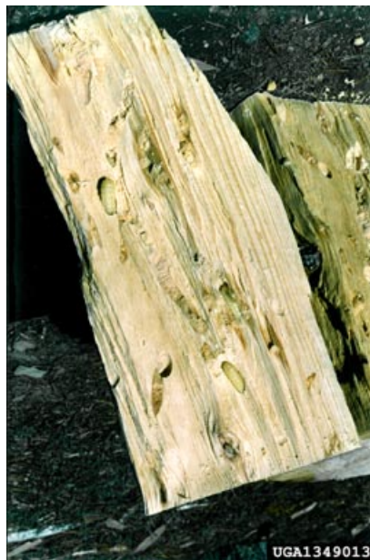
Figure 1. Wood Infested with Sirex noctilio Larvae. Paula Klasmer, Instituto Nacional de Tecnologia Agropecuaria, www.forestryimages.org
