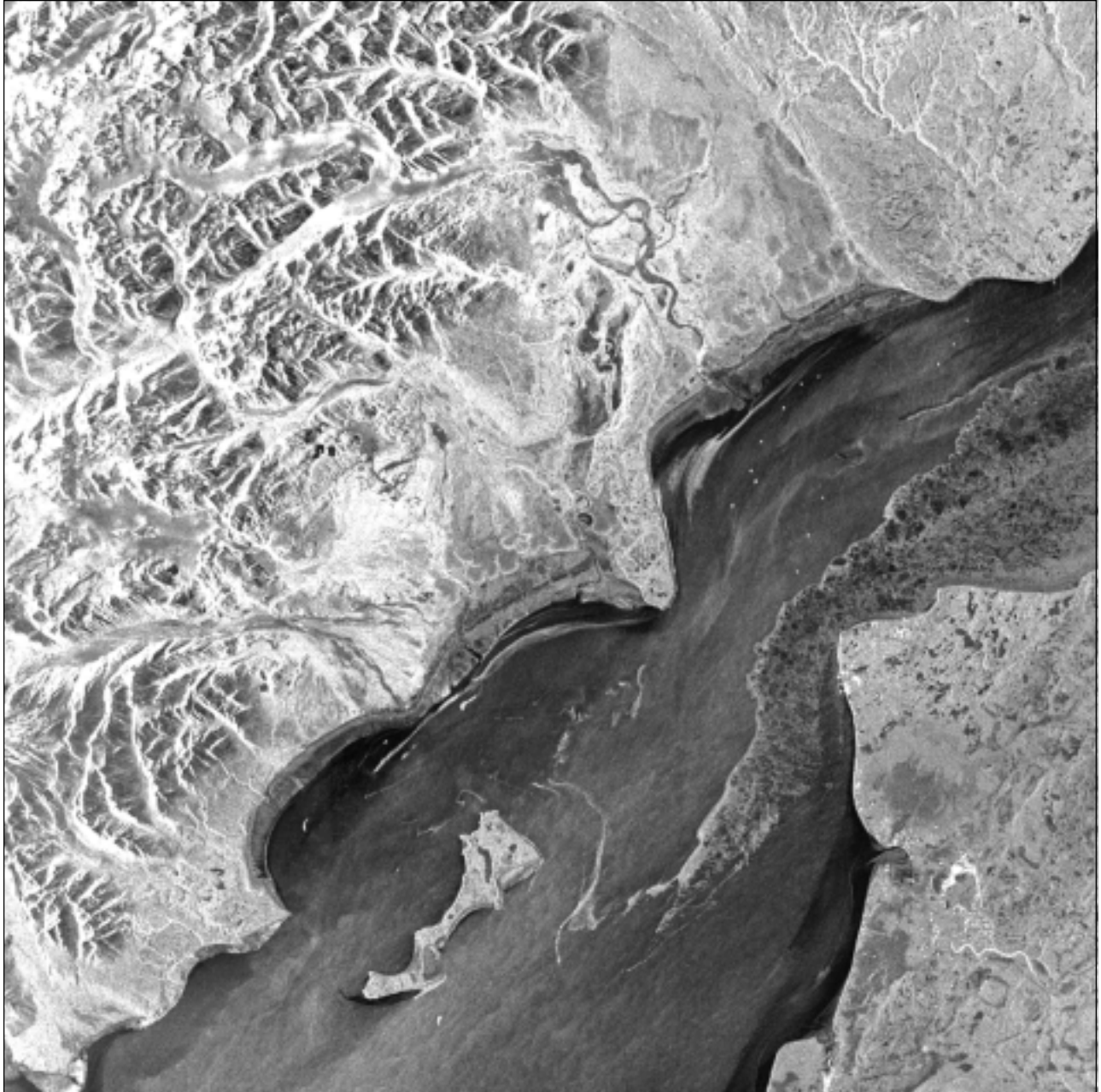
Figure 14. Radarsat-1 SAR imagery showing the Forelands area of Cook Inlet at near low tide on December 30, 1998. The region appearing stippled along the East Foreland is 6 to 10 tenths young and first-year thin sea ice. Tidal flats are visible along the northern shores with streaks of 5 to 7 tenths new ice forming just offshore in Trading Bay and Redoubt Bay. The bright white specks in three distinct rows that appear in the water north of the Forelands are oil production platforms. [Image copyright by Canadian Space Agency (1998); used by permission.]
