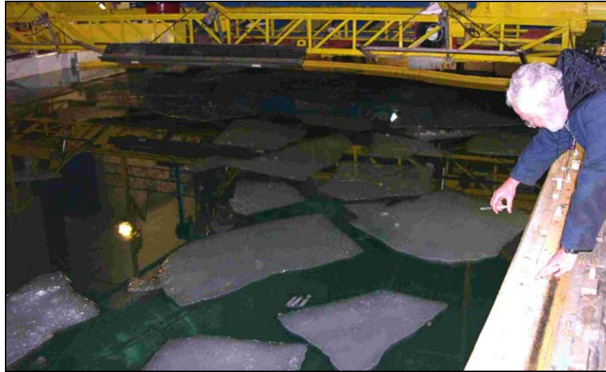
Ian Buist, SL Ross Environmental Research Ltd., applies herding agent around the periphery of a test slick among broken ice in CRREL's test basin. (Photo courtesy of Ian Buist)
