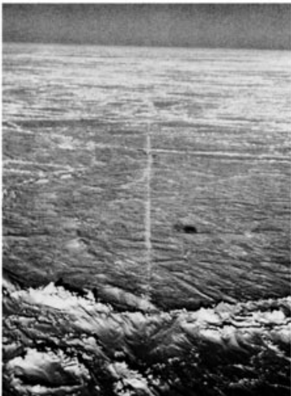
Figure 4. Aerial view of ~1.0-km-long survey line. The line extends from multiyear sea ice, in the foreground, to first-year sea ice in the background. The dark spot to the right of the survey line is the shadow of the helicopter from which the photo was taken.
