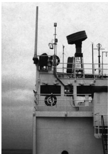
The aft port bridge of the Polar Sea , showing the triple-headed air sampling manifold leading into a rear window of the bridge superstructure.
