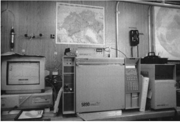
Equipment used on the Polar Sea to analyze DMS samples. The system consists of a gas chromatograph with a sulfur chemiluminescence detector.
