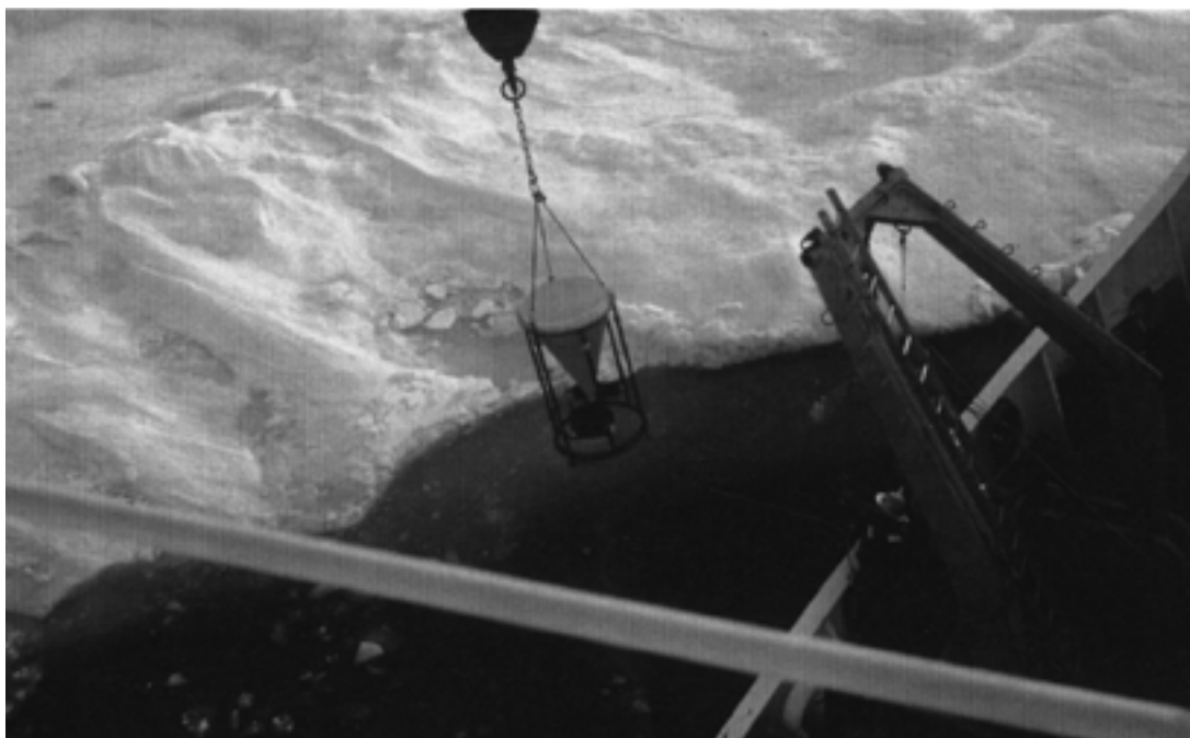
Sediment trap being lowered into the water to collect samples for contaminant chemistry studies.
