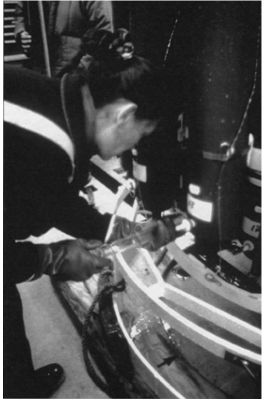
Fiona McLaughlin drawing water samples from the Niskin bottles for chemistry analysis on the Louis S. St-Laurent
