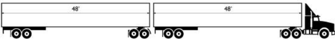
Turnpike Doubles – a tractor pulling two 48' foot trailers
