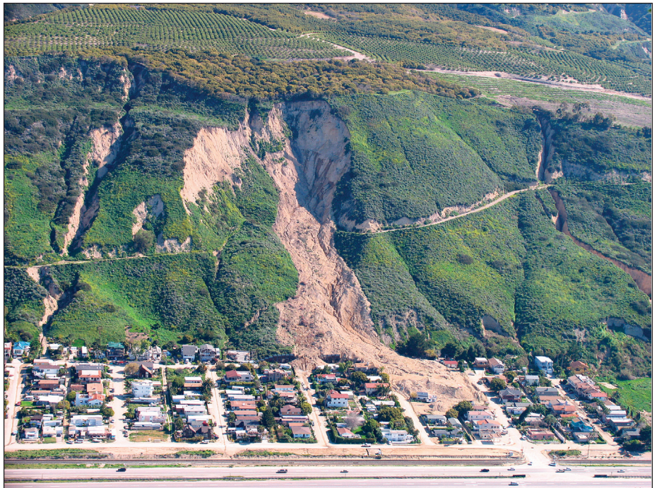
View of the La Conchita landslide taken March 16, 2005. The lightest-colored, exposed rock to the left of the center of the photo is the main scarp of the 1995 slide. The southeast part of the 1995 deposit (central part of photo; it extends into a housing development) remobilized in 2005. Photograph by Jonathan Godt, USGS. A report on the La Conchita landslide is available online: http://pubs.usgs.gov/of/2005/1067
