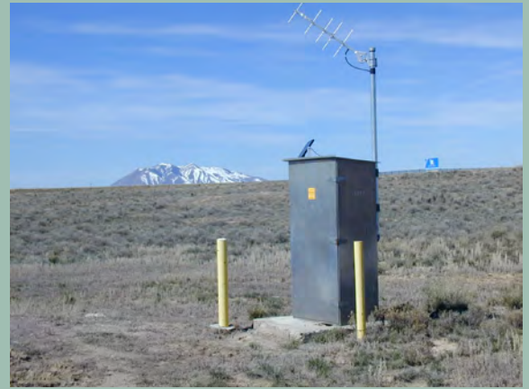
Real-time monitoring well that is part of the USGS Ground-Water Climate-Response Network in Idaho (photograph by Matthew Gilbert, USGS).
