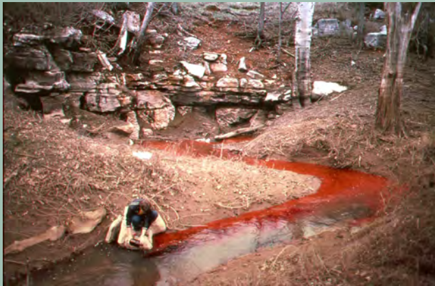
Rhodomine dye is injected in a stream to trace water movement through a karst aquifer (photograph by Charles Taylor, USGS).
