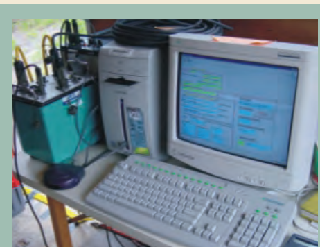
Field testing and development of a web-enabled, earth-resistivity tomography monitoring system (photographs by Kamini Singha, USGS).
