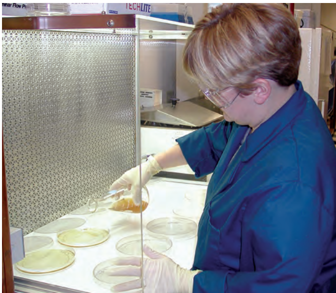
OWML laboratory technician analyzing a water sample for coliphage using a single-agar layer technique
