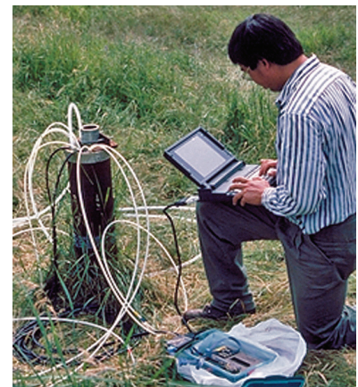
A multi-level monitoring well is set up in a fractured rock aquifer in New Hampshire
