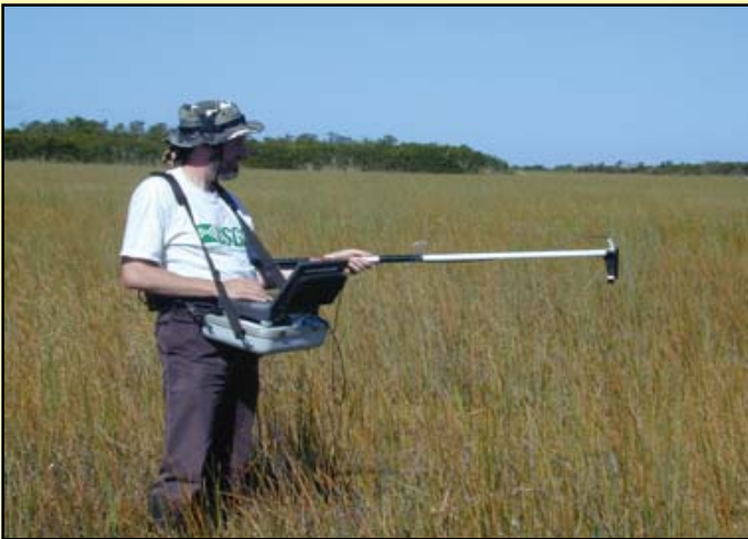
Figure 3. A library of South Florida land cover spectra is being built using handheld and laboratory spectroscopy.
