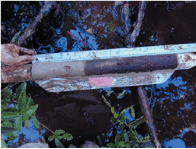
Figure 2. A coring device is used to extract soil from a mangrove ecosystem to help USGS scientists reconstruct the vegetation history of the site. The extracted core shows mangrove peat deposited beneath a sand layer.
