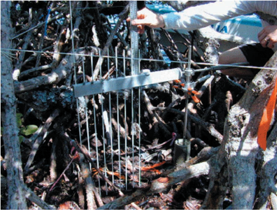
Figure 4. Measurement of soil elevation change in a mangrove ecosystem in Belize using a rod surface elevation table.
