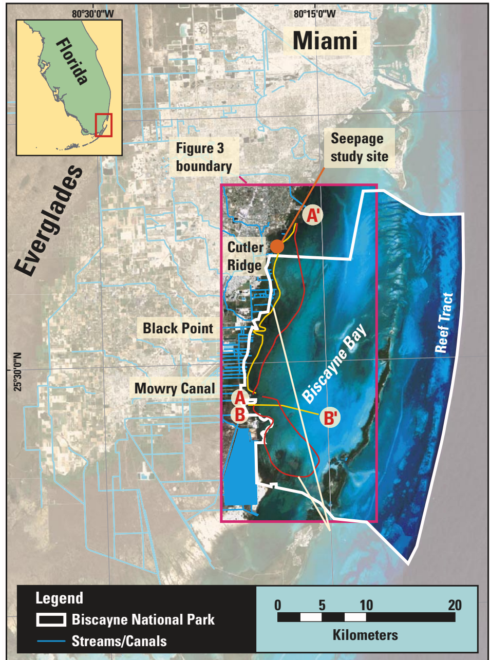
Figure 1. Landsat TM image of south Florida showing Biscayne Bay and Miami. Water-column ^{222}\text{Rn} and streaming resistivity survey track lines (A-A' and B-B') as well as the electromagnetic seepage meter site (●) at Cutler Ridge are identified.
