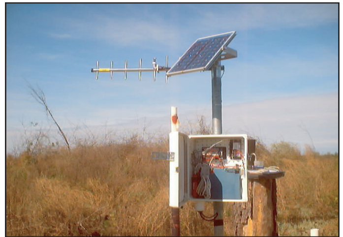
Figure 6. Water-level monitoring equipment (photograph by Ralf Montanus, U.S. Geological Survey).
