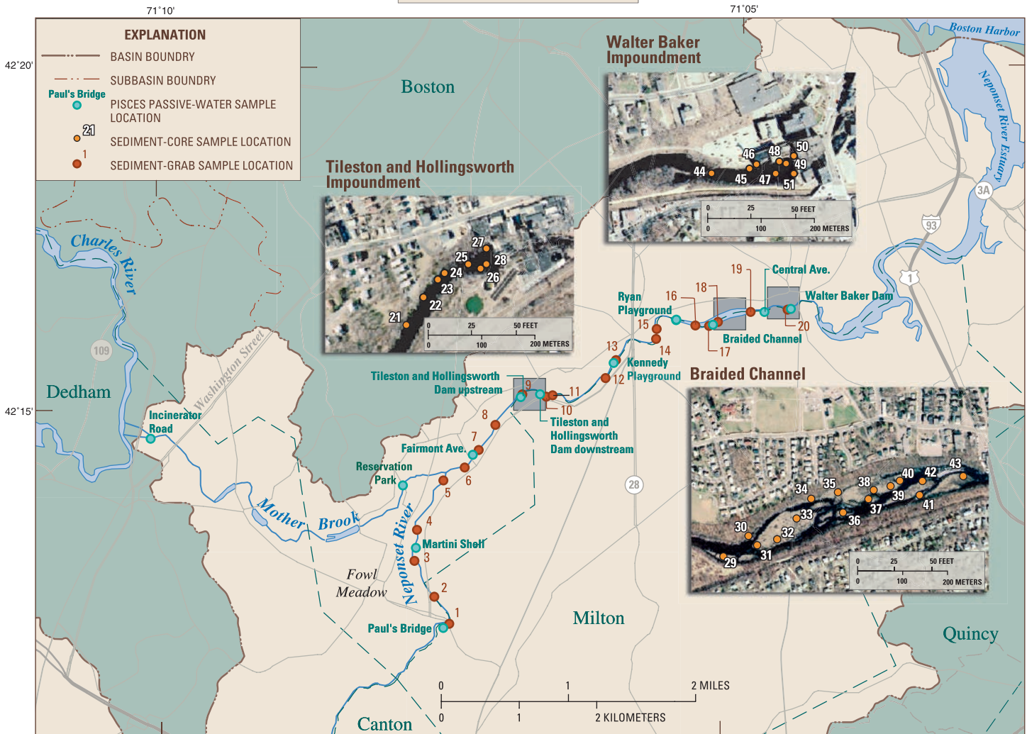
Figure 1. Sediment-grab (top 2–4 in. of sediment) and sediment-core (5–50 in., depending on the total depth of the sediment) sampling sites and location of passive-water-sampler (PISCES) deployment, in the Neponset River of Massachusetts.
