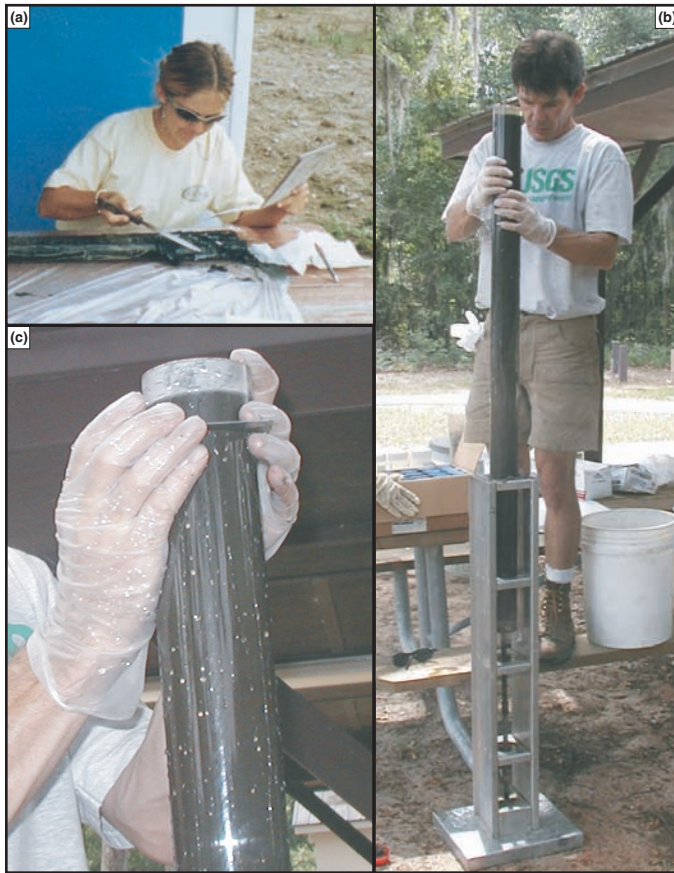
Figure 2. U.S. Geological Survey personnel (a) describing a gravity core, (b) placing gravity core in core extrusion stand, and (c) slicing a subsample from a gravity core (photographs by Barbara J. Mahler, U.S. Geological Survey).
