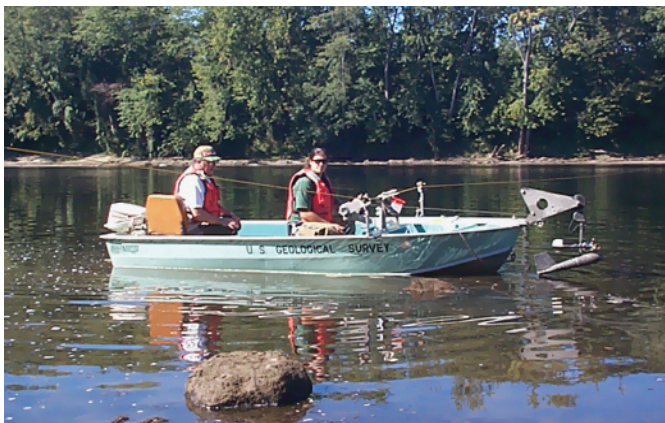
Figure 2. The USGS measures discharge on the Connecticut River at Montague City, Massachusetts, 2001.
