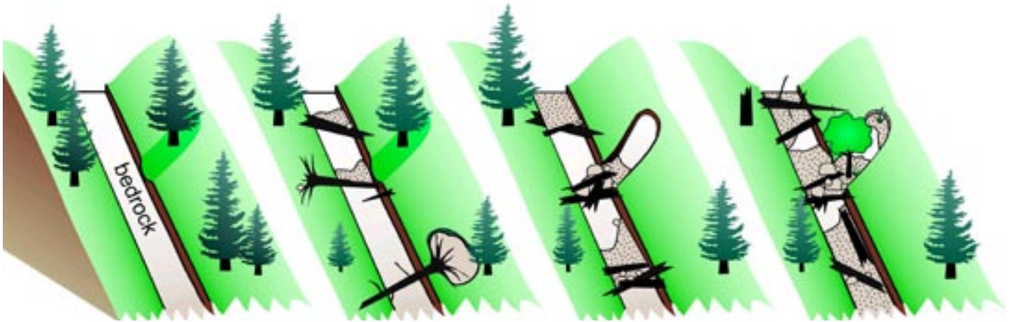
Figure 4. Conceptual illustration of the changes in channel morphology in steep headwater streams, based on the time since the previous debris flow.
