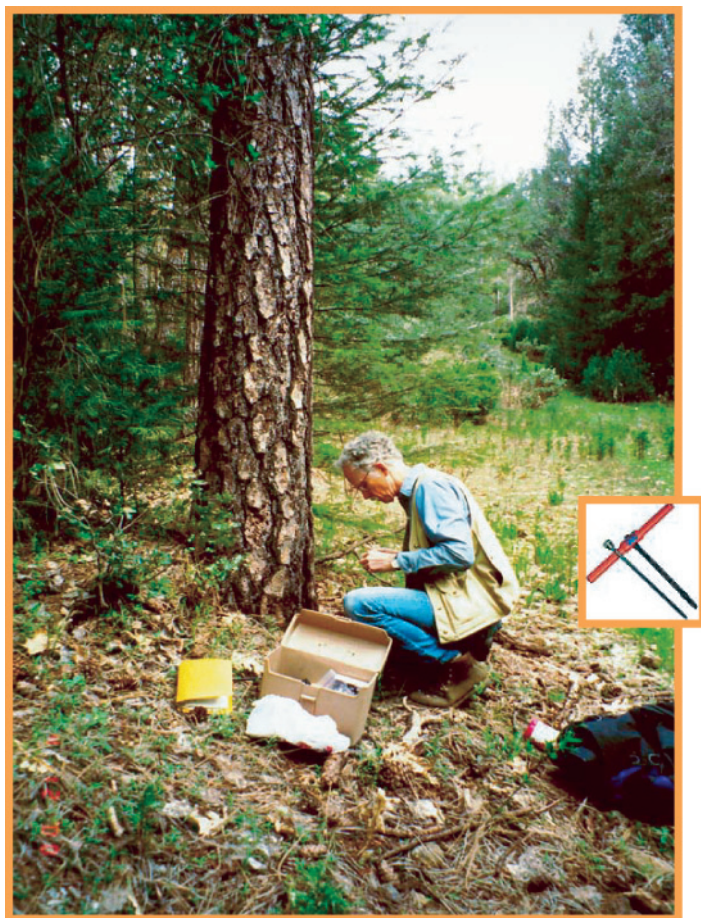
Cores were extracted from ponderosa pine using an increment borer (inset). Usually more than one core was extracted from each tree in order to measure the chemical variability between cores within a tree.
