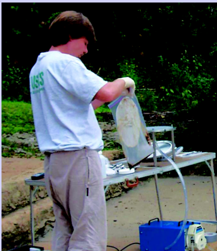
USGS hydrologist Marcus Gary collects suspended sediment at Main Barton Spring. The sediment has been removed from the filter by massaging and has collected in the bottom of the locking plastic bag. The blue peristaltic pump and the stainless steel filter holder are visible in the background.
