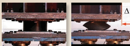
Base isolators in laboratory tests—(left) undeformed isolator, (right) deformed isolator with sizeable horizontal displacement ( \Delta ). Such displacement of isolators prevents large displacements of floors of the building above.
