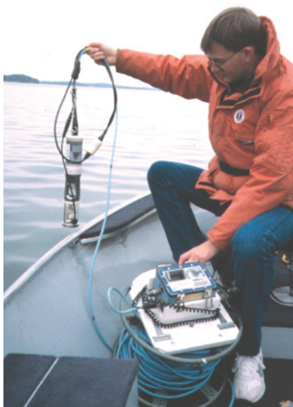
Figure 4. Measurement of lake water-quality profiles with a multi-parameter water-quality instrument.
