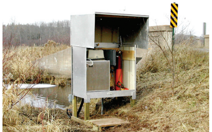
Figure 7. Typical U.S. Geological Survey recording streamflow-gaging
