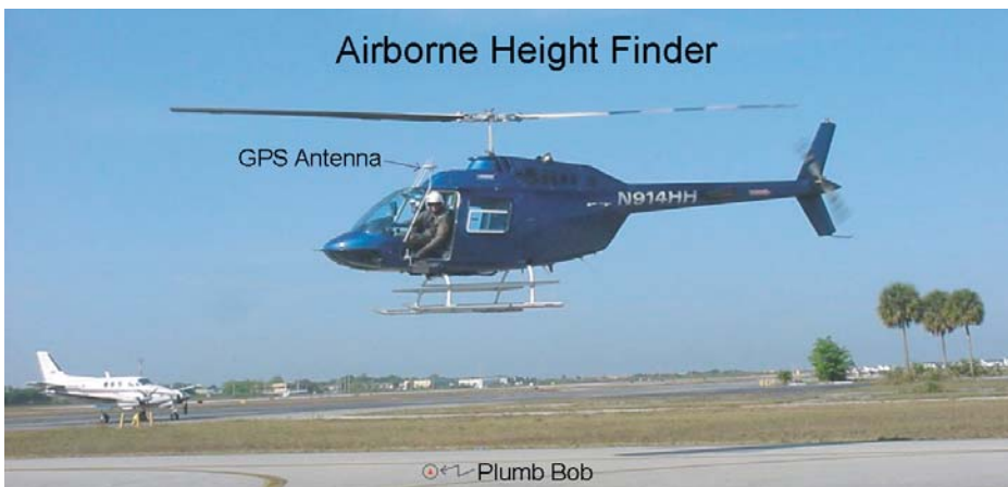
Figure 3. Operation of the Airborne Height Finder is demonstrated. The plumb bob is deployed from the helicopter to the surface being measured.
