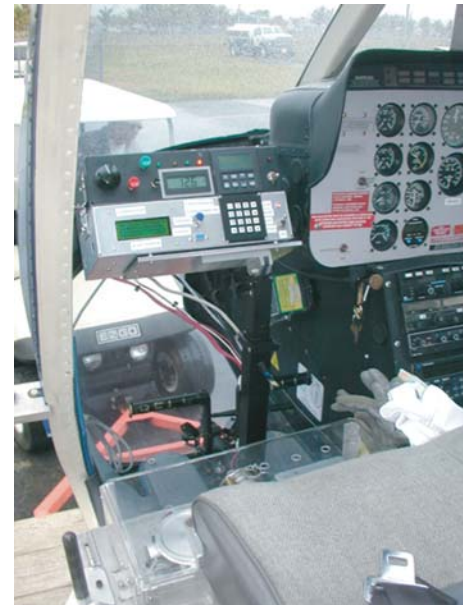
Figure 4. The Airborne Height Finder is operated using the USGS-developed electronic controller and interface.
