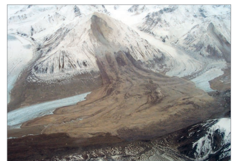
This huge landslide from an unnamed 7,000-foot-high peak in the Alaska Range, less than 10 miles west of the Trans-Alaska Oil Pipeline, was triggered by the 2002 Denali Fault earthquake. The fault rupture offset the ice of the mile-wide Black Rapids Glacier, in the foreground, which the landslide subsequently covered.
