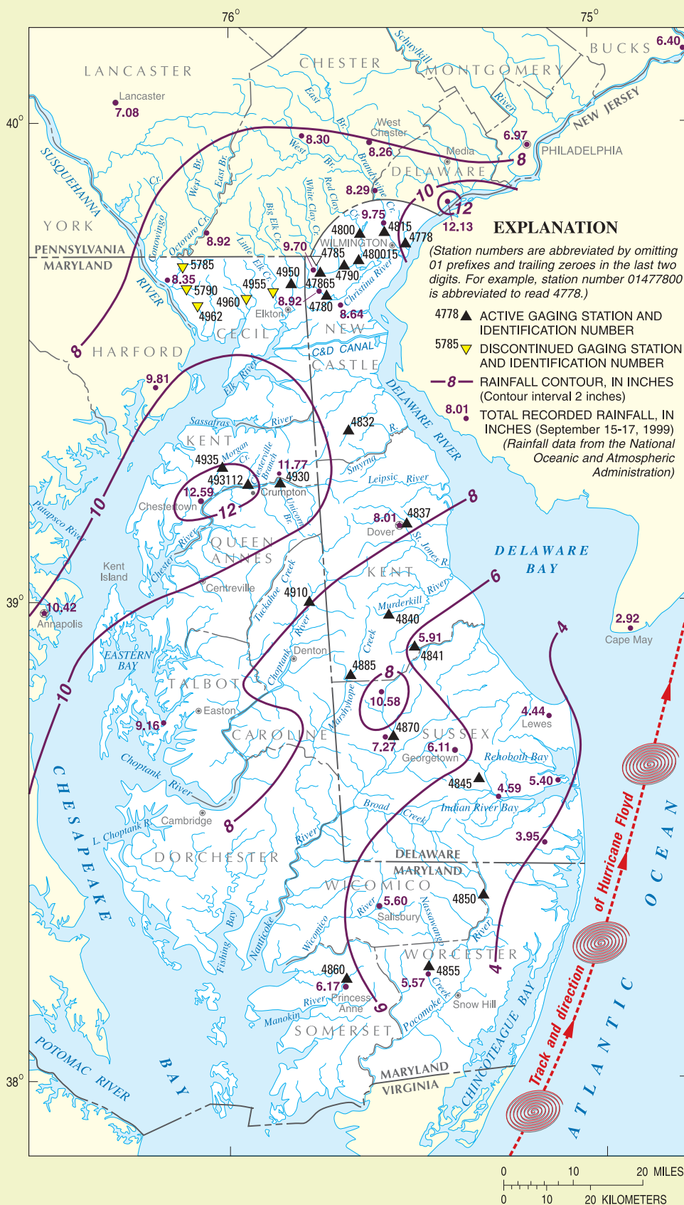
Figure 3. Location of active and discontinued streamflow-gaging stations in Delaware and the Eastern Shore of Maryland, rainfall distribution, and track and direction of Hurricane Floyd, 1999. (modified from Tallman and Fisher, 2001)
