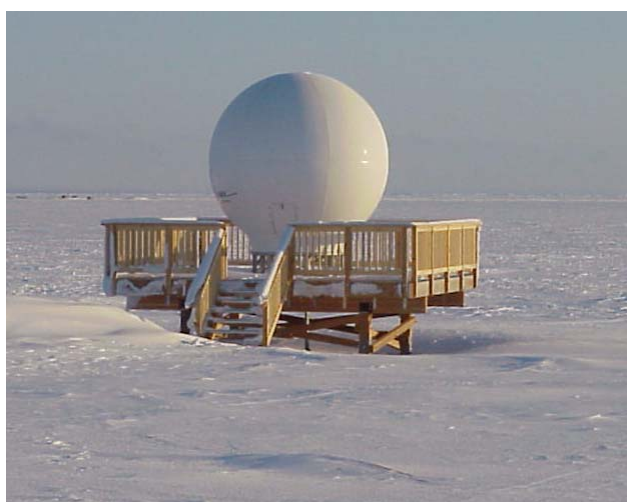
Figure 1.2. NOAA NESDIS platform and antenna dome for downloading polar orbiting satellite data at the Barrow Baseline Observatory.
