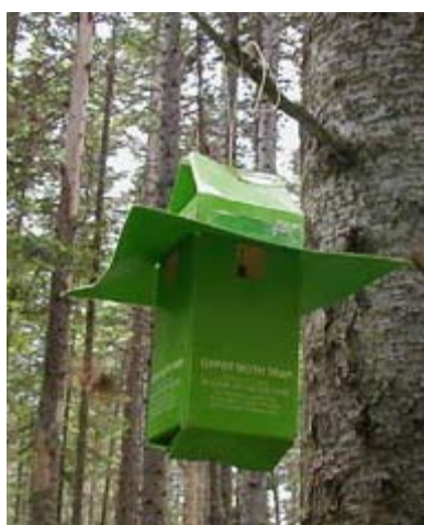
Figure 3. Modified milk-carton type trap baited with pheromone for the detection of Dendrolimus superans [Image from A. Tyskalov, http://www.forestproject.ru/web2/pests/pests.htm ]
