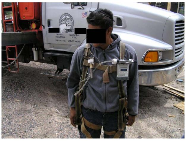
Figure 2. Cutter/Roofer with sampling equipment.
