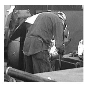
Figure 7. Welder Welding Piece in Flexed Posture Despite Positioner
