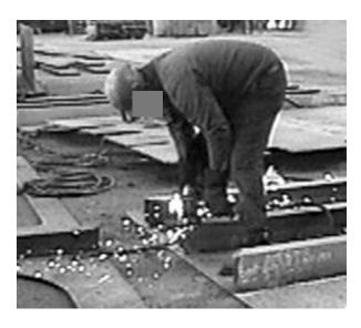
Figure 8. Panel Line Worker Grinding
