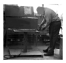
Figure 10. Manhole Assembler Clamping Hatch
