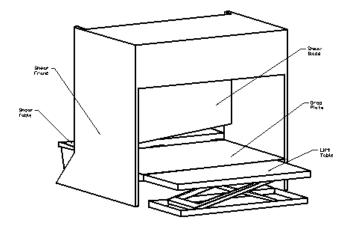
Figure 12: Shear with Lift Table in Up Position
