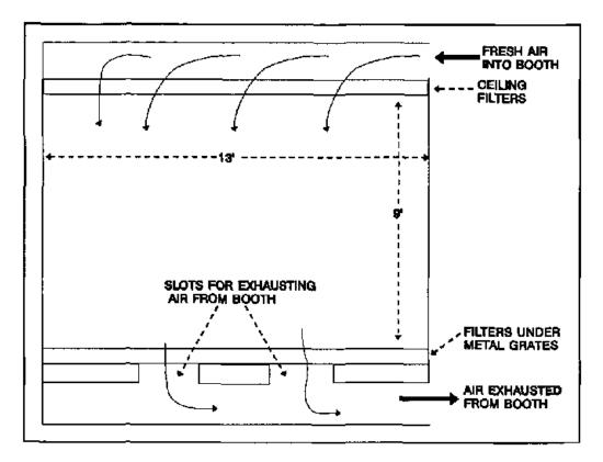
Figure 3 Schematic of spray painting booth
