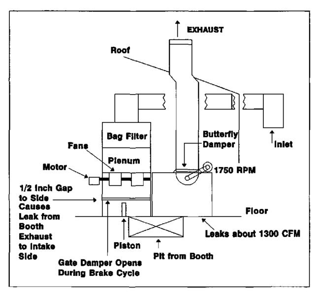
Figure 4 View of the paint booth's ventilation systems
