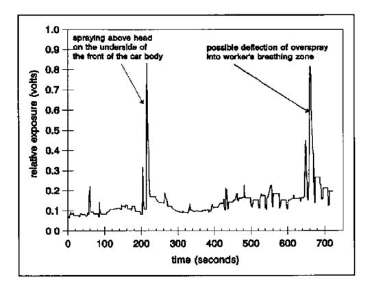
Figure 7 Relative exposure during spray painting in downdraft spray painting booth The front of a car body was being painted
