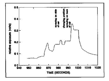
Figure 11 Relative exposure while spray painting car at the vehicle preparation station
