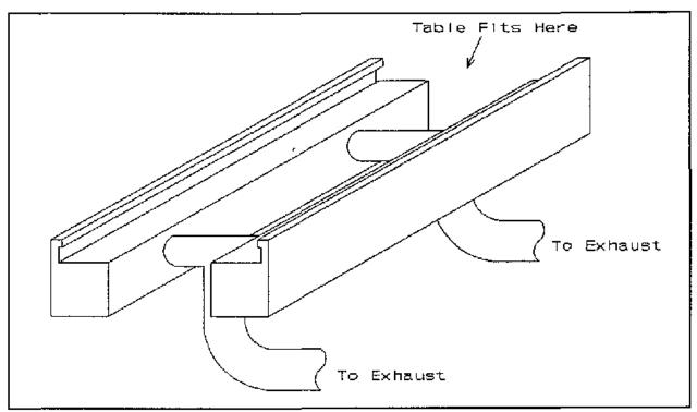
Figure 3 Diagram of local exhaust ventilation hood
