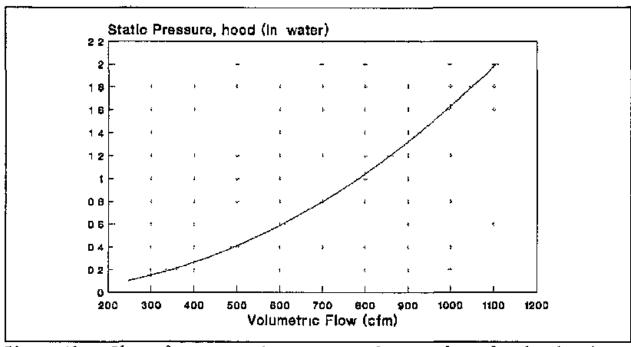
Figure Al Plot of pressure drop versus exhaust volume for local exhaust ventilation hood
