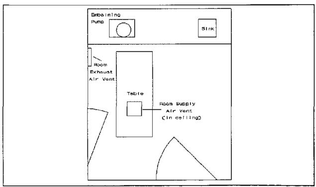
Figure 2 Diagram of isolation room
