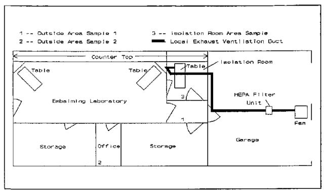
Figure 1 Diagram of mortuary laboratory area
