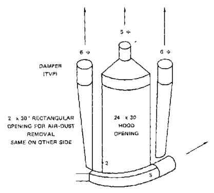
NOTE. All four above units to be mounted on hood around the 24 ix 30 liopening
