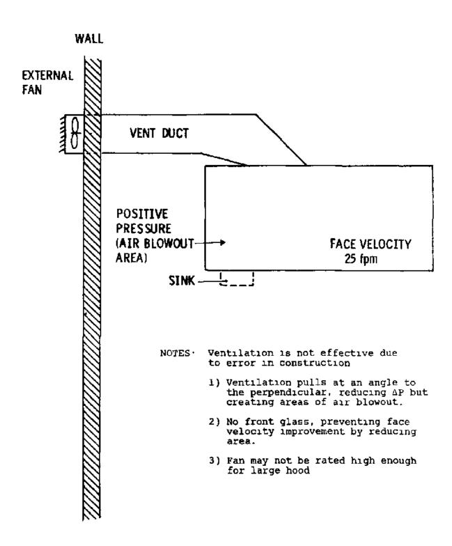
Figure 36. Diagram of laboratory hood.
