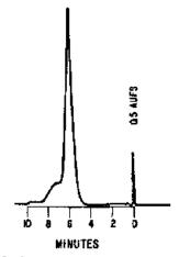
Figure 1. HPLC chromatogram for injection of 4.6 µg of formaldehyde-2,4-distrophenythydrazone (equivalent to 1.08 ppm formaldehyde in air, for a 20-L air sample)
