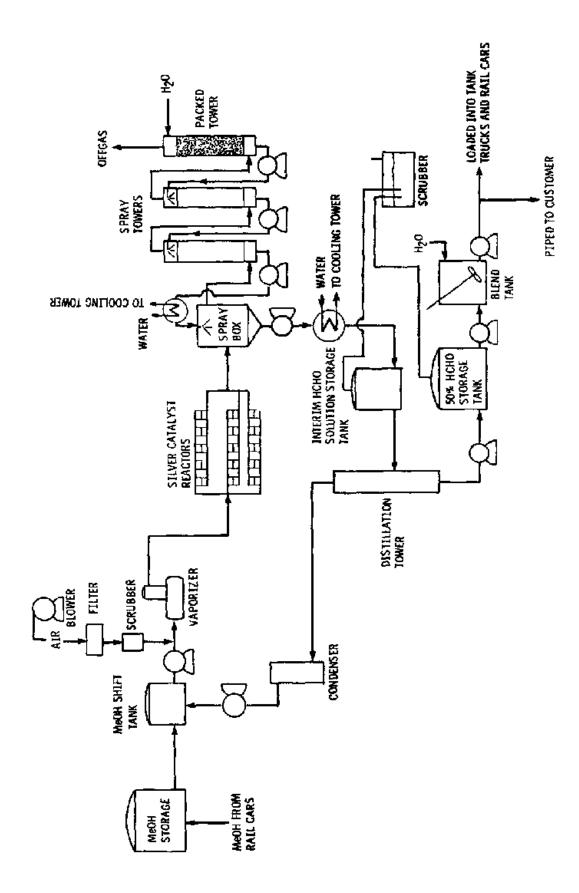
Figure 3. Schematic of Hampton formaldehyde process.
