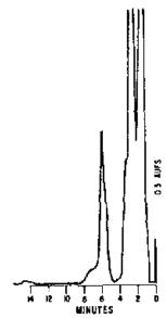
Figure 3 HPLC chromatogram for a field sample at a location where termaldehyde is used as a raw material. The sample was determined to represent 0.85 ppm formaldehyde in air.
