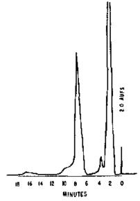
Figure 2. HPLC chromatogram for injection of sample resulting from collection of 122 μg of formaldehyde (4.96 ppm for a 20-L sample) on a 2,4-DNPH coafed slica gel tube, as described in the Experimental section.
