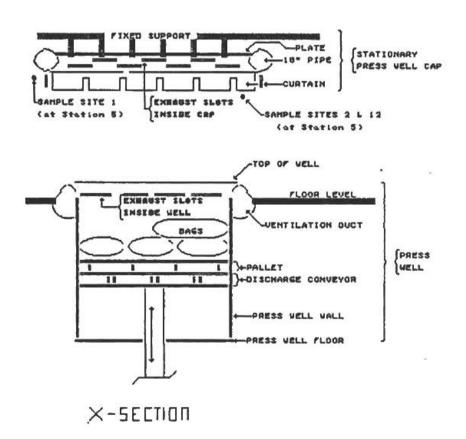
Figure 2: Press Well - Palletizing
