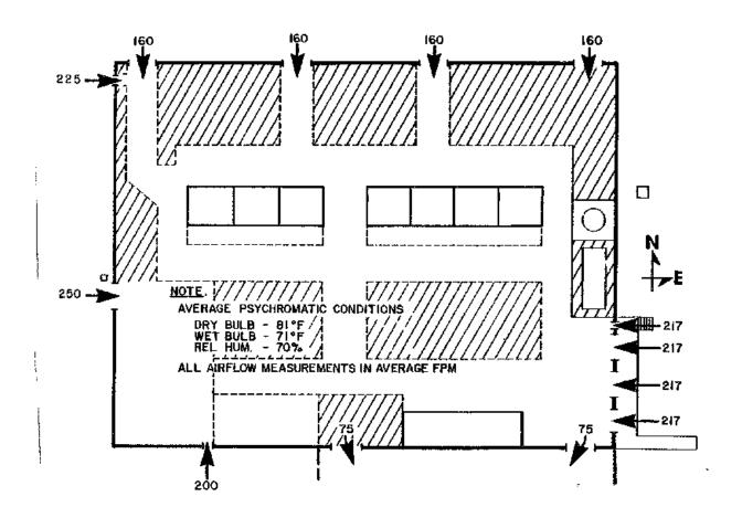
Figure 27. General ventilation through wall openings
