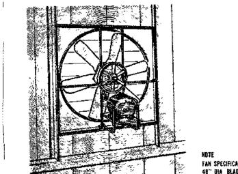
NUJE FAN SPECIFICATIONS 3HP, 535 RPM, 48" DIA BLADE, 25400 CFM, ½IN.SP.
