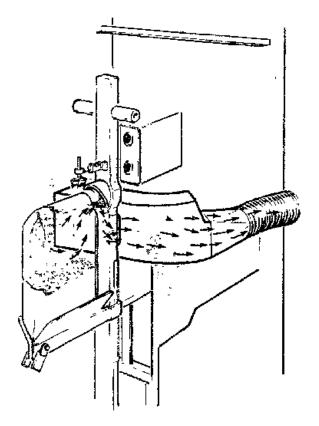
Figure 14. Typical bagging station exhaust ventilation air flow
