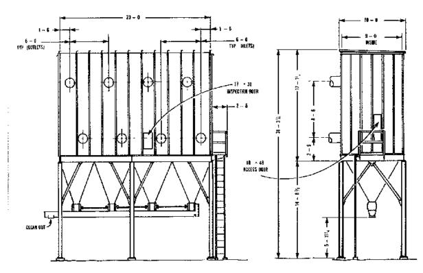
Figure 7. Dust collector details
