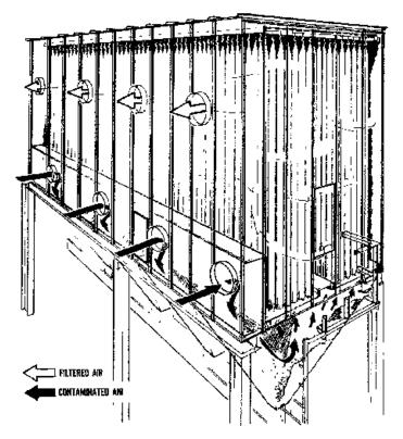
Figure 6. Dust collector air flow
