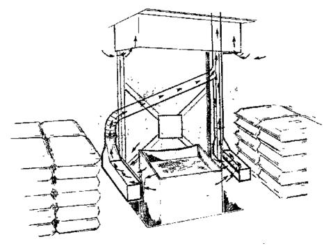
Figure 10. Typical batching station air flow
