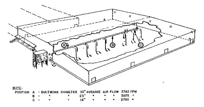
Figure 5. Exhaust system ductwork
