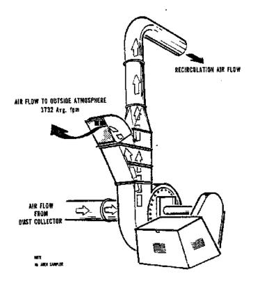
Figure 9. Dust collector blower air flow
