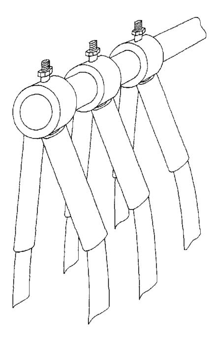
Figure 3 TWECO Roto-grounds Mounted on a Rotating Shaft.
