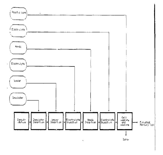
Figure 7. Cell Assembly - Process Flow Diagram.
