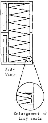
Figure 18. Charcoal Filter Rack Configuration.
