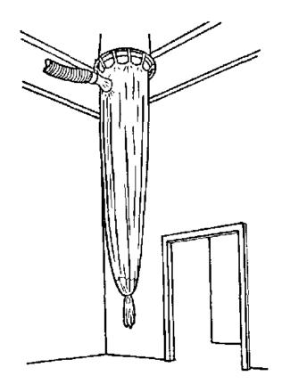
Figure V-17. Filter Bag for Removing PMA from Exhaust Air.
