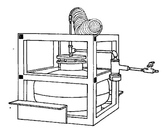
Figure V-6. Mercury Storage Container.
