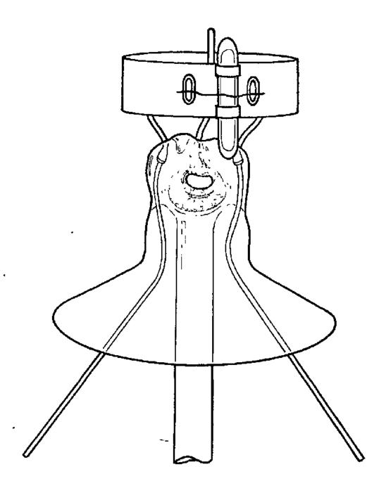
Figure V-3. Mount Assembly with Mercury Pill.
