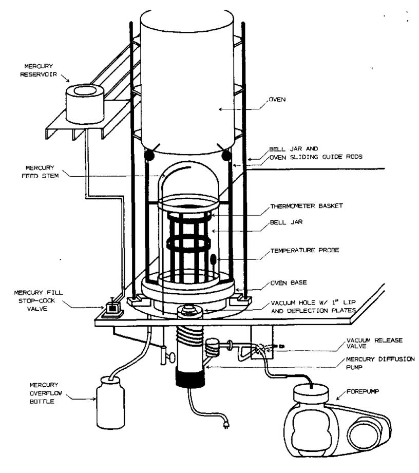
Figure V-5. Schematic Diagram of the Mercury Filler.
