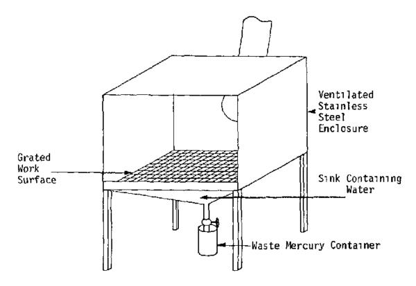
Figure VI-2. Ventilated Work Station with Grated Surface
