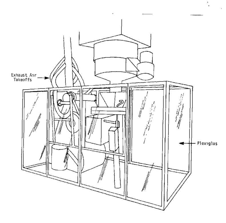
Figure V-10. Plexiglas Machine Enclosure.
