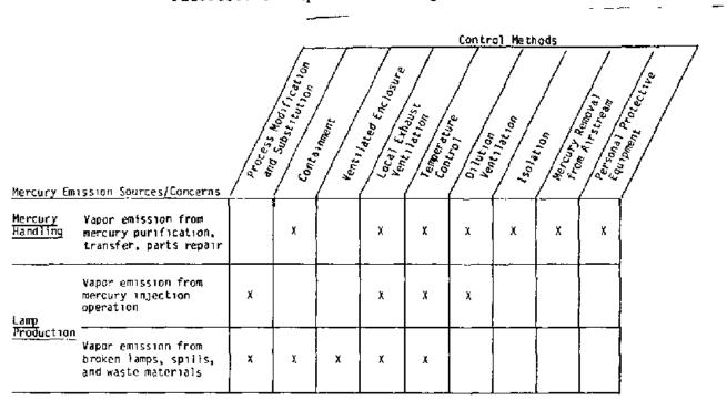
Mercury Emission Sources and Control Methods for the Fluorescent Lamp Manufacturing Industry
