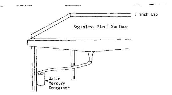
Figure VI-1 Work Station with Drainage Trough
