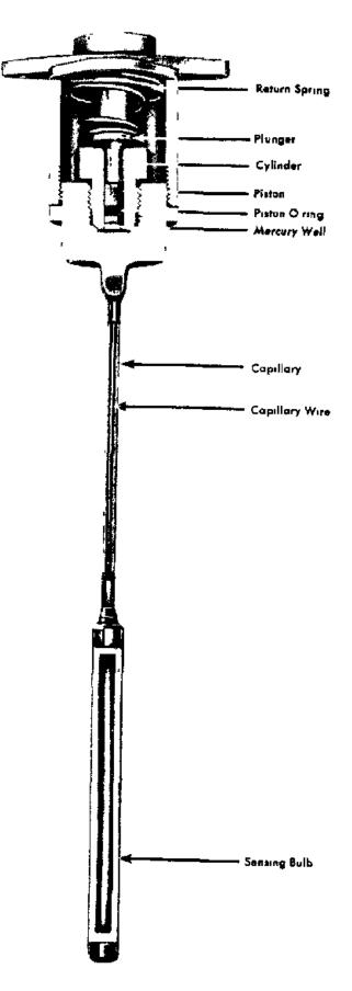
Figure IV-1. Temperature-Sensing Instrument.
