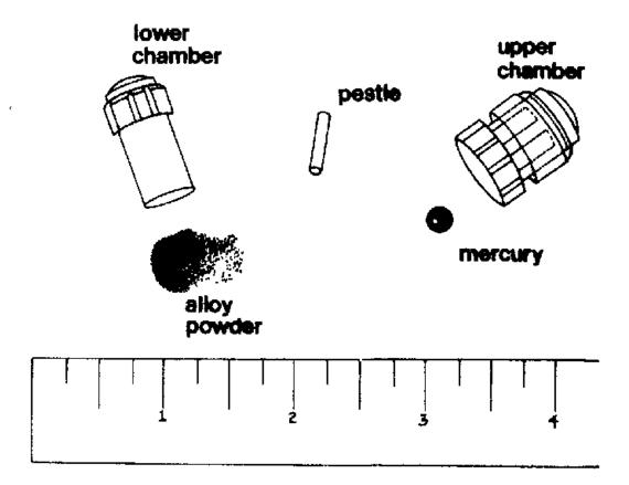
Figure V-2. Dispersalloy  $^{R}$  Dispos-a-cap Component.
