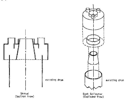
Figure V-19. Schematic Drawing of Drum Loading Hood. Reference. Plant drawing from site visited.
