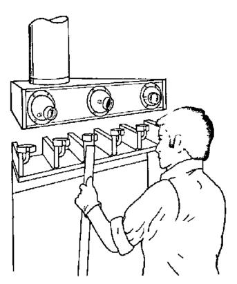
Figure V-21. Adjustable 2-Inch Supply Air Vents.
