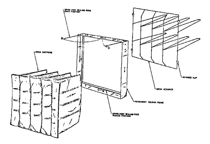
Figure V-24. Fiber Filters for Particulate Removal.
