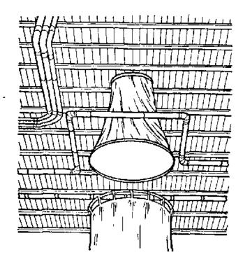
Figure V-15. Shroud Over Exhaust Machine.
