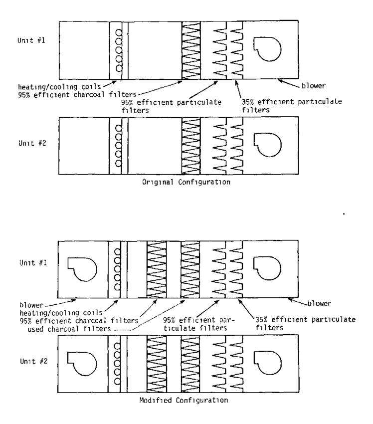
Figure V-25. Original and Modified Air Handler Configurations.
