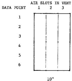
Note: The width of the vertical air slots varies from 3.25" to 4" and results in different data point areas.
