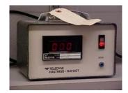
3.1.2. Teledyne-Hastings Raydist mass flow meter, Model NAHL-25, or equivalent
