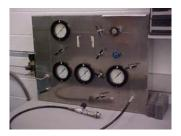
3.1.3. A test stand incorporating four Weksler calibrated pressure gauges (two 0-10,000 psig and two 0-3,000 psig), or equivalent. NOTE: Calibrated pressure gauges must be selected so that required readings fall near the midpoint, and never within the first or last 10%, of the gauge's pressure range.
