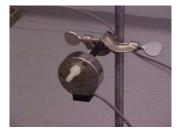
Temperature compensated pressure transducer (Validyne Engineering Model No. DP45) or equivalent.
