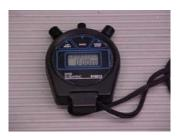
3.1.7. Timer, Digital stopwatch, calibrated to hundredths of a minute (Cronus Precision Products, Inc.) to hand carry. or equivalent.
